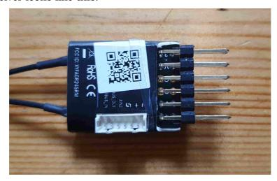
Firstly, remove the case and cut the servo connector pins off using very sharp side cutters. De-soldering and pulling out the pins is possible but not necessary and increases the risk of damage to the board. Carefully crop the ends close to the PCB.
