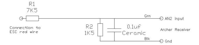
The resistor values shown are those used in the FRSky divider for a 3S battery. Calculations of values for other batteries are given later in this article. I use 1/4 watt metal film resistors but you can use as small resistors as you like (or can manage to solder!) as heat dissipation is very low in this circuit. I prefer metal film resistors which are usually robust and stable.
