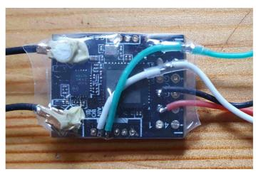
Part of the heat shrink can be cut away on the underside to access the push button.
