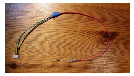
We could shorten the black and green wires and have a longer red wire to bring the resistor and capacitor closer to the receiver if we wish.
