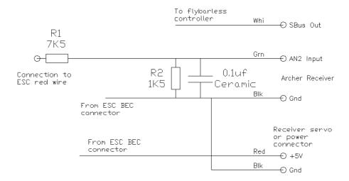
In this diagram I have shown the ground connected to both the smartport and servo connectors and the +5V connected only to the servo connector. We can connect both + and - to both connectors or only to the servo connector as we wish.
