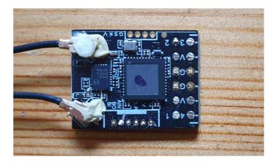
Wires can now be soldered directly to the pads. In this one you can see the green and white wires have been extended about 2cm. The blue heat shrink package contains the resistor and capacitor for the voltage divider.
