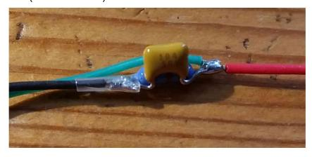
Solder the 7K5 resistor R1 to the other end of the wire, put heat shrink sleeve over the soldered ends and a larger piece over the capacitor and resistor.
