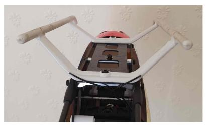
This gets the antennae away from the carbon fibre frame and sets them at approximate right angles to each other. It gives good range check results. This should not be done on metal or carbon fibre legs.
