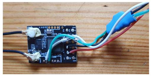
Note that the push button and indicator light are underneath the board in this orientation. Now is a good time to bind and test the receiver.
