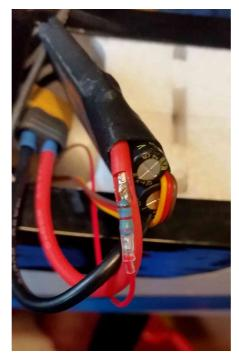
Cover the soldered joint and the resistor with some PVC insulating tape. PVC insulating tape is not the ideal solution, so if you find something better let me know! If you are prepared to disconnect and re-connect the power wire at the battery connector socket you can use heat shrink sleeve instead.
