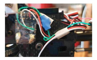
The receiver can be mounted on its other side to retain access to the push button. However the orientation shown gives the flattest surface for sticking with double sided tape.
