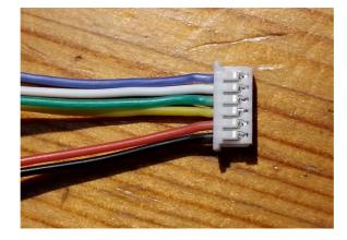
We only need the green (A2 telemetry input) and black (ground). Clip the unused wires close to the connector or, alternatively, lever up the plastic latches which retain the unused crimps with the tip of a craft knife, watchmakers screwdriver or similar and remove the crimps from the housing.
