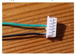
At the other ends of the black and green wires solder the 1K5 resistor R2 in parallel with the 0.1uf ceramic capacitor. Shorten the black wire so the resistor and capacitor lie along the green wire.
