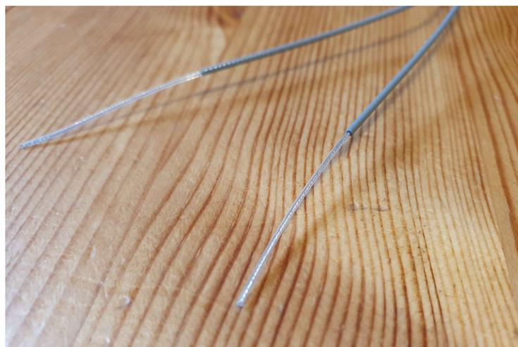
No installation is perfect, but our objective is to get the end bits straight, as far away from the rest of the receiver, wiring, servos or power installation as we reasonably can and, if possible, approximately at right angles to each other. The idea of having two antennae is that if the signal is poor in one it might be better on the other.
