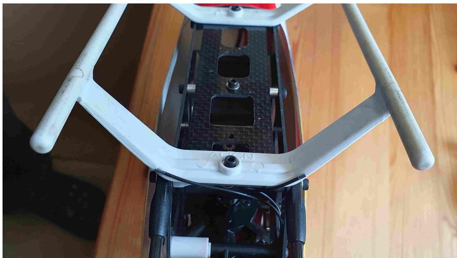
The legs are well away from the chassis and approximately at right angles to each other. Of course this would not be a good idea with metal or carbon fibre legs.
