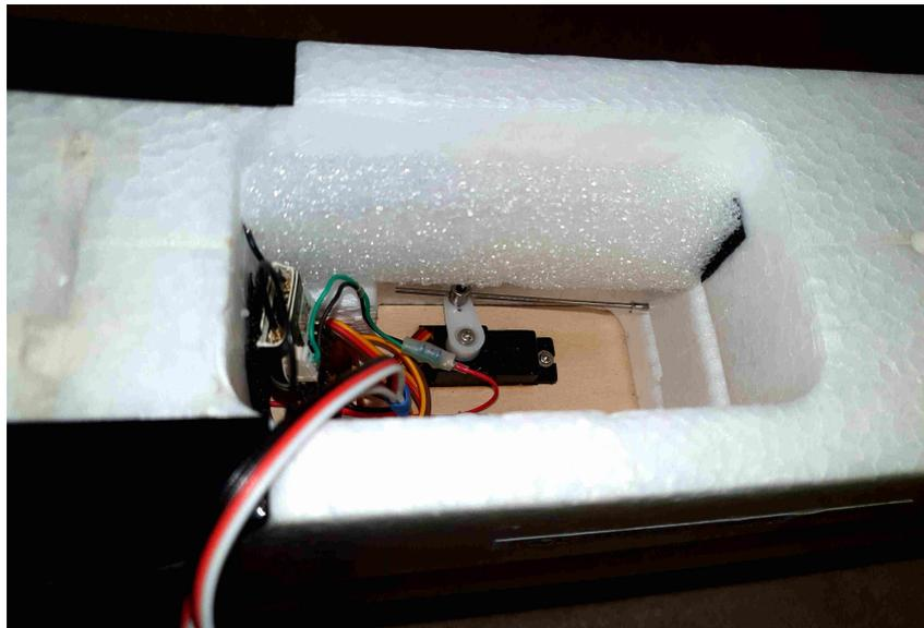
A small piece of self adhesive velcro “hook” material on the right hand side of the picture helps to keep the foam in place.
