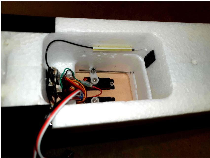
The picture above shows a piece of plastic straw holding an antenna in a Century Models Riot. The end of the “whisker” extends further into a hole I made in the expanded polystyrene. In this way the antenna is kept away from the wiring and the steel wire pushrods.
