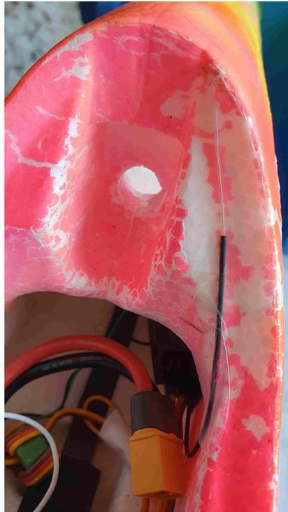
When fitted, the canopy presses the antenna against the bulkhead. The other antenna (not visible) is in a plastic tube glued to the inside of the fuselage running back at an angle directing it away from the servo wiring.
