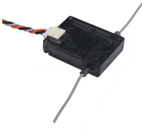
I am unclear whether the two “whiskers” on these devices are separate antennae or two parts of a dipole but the unit should be considered as a single antennae and oriented with the wires sticking out as in the picture and at right angles to those on the primary receiver.
