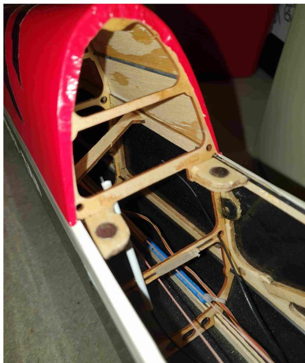
Note this model is constructed with wood re-enforced with carbon fibre rods and strips.
