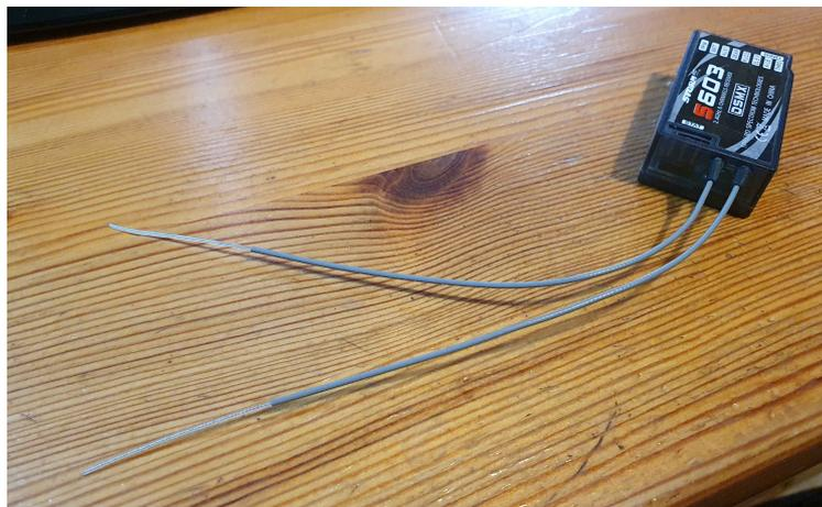
These are pieces of coaxial cable with about 30mm of the outer conductor stripped away at the end. The type and length of the cable and the amount stripped away may be matched to the type of receiver so if you damage an antenna get a proper replacement. The exposed “whisker” does the actual receiving.
