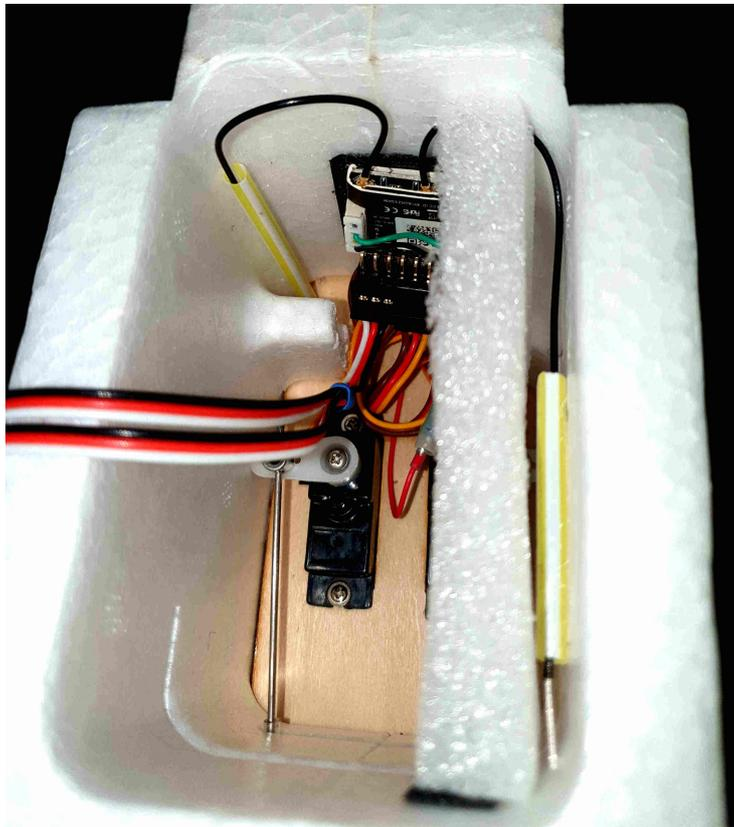
This keeps it a short distance from the receiver and wiring. I could have made more effort to place it further away from the receiver but in this aircraft it works fine. I would not want it any closer though.
