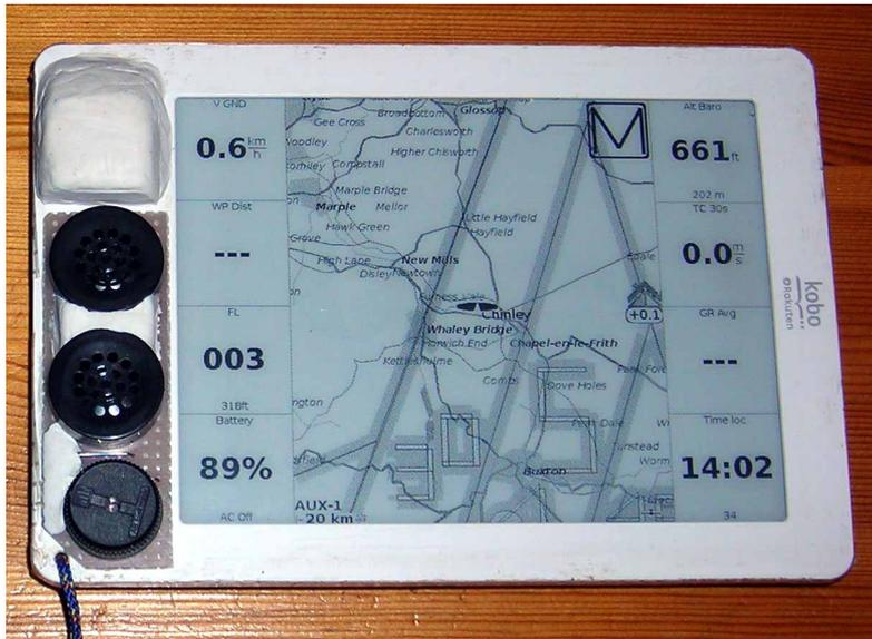
The switch, resistors and miniature speakers are mounted on a piece of stripboard fixed to the front of the Kobo using double sided foam tape. In the unit shown the resistors are embedded in Sugru as is the GPS module. The pin with common connection to the switch is bent sideways and connected to a short piece of wire before fitting to the board.
