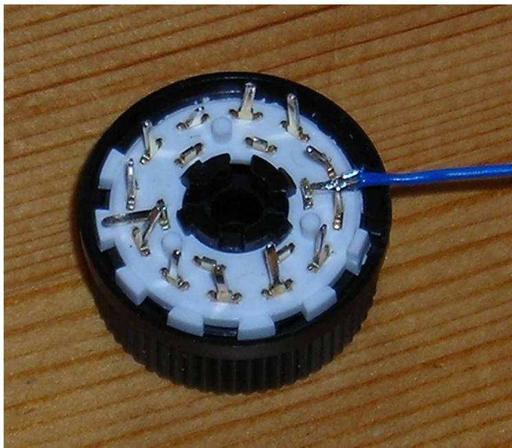
Four of the pins are bent slightly inwards to make the circular pattern fit the stripboard, and the switch carefully aligned to get the required function. This system is surprisingly robust and I have used one taped to my helmet to adjust the volume of a radio headset. It can easily be operated with fairly thick flying gloves and clicked to a specific volume setting even at when no transmission can be being heard.
