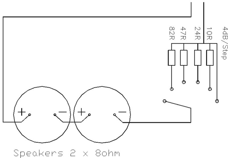
The switch I use is a 2 pole 6 way PCB mounting switch AB 417 Conrad part No. 705683-62 . The resistor values in the diagram give a change of volume of about 4dB per step with a 16 ohm speaker. The bottom position is completely off.
