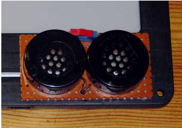
At the top of the board a small slide switch which was mounted on the stripboard to cut the speakers can be seen. It is not intended to be used in flight but I wanted to be able to cut the audio when using the unit on the ground for retrieve or rescue purposes.
