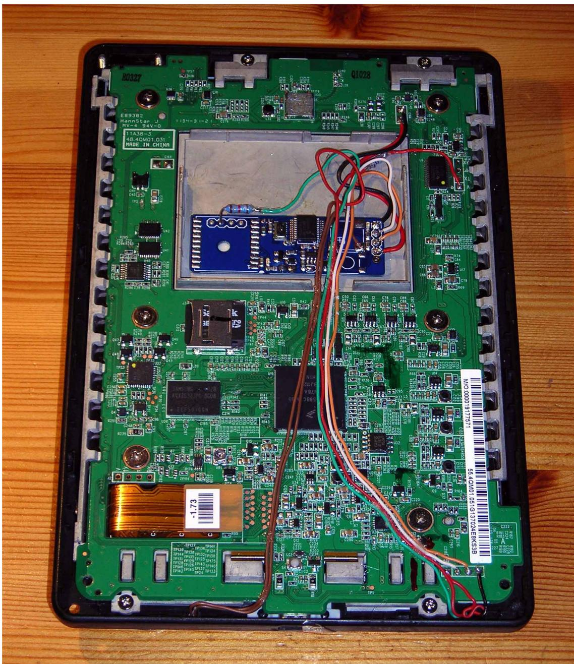
To ensure the wires were not crushed the wires had to be very carefully routed and webbing strategically removed from the inside of the back case. Inside the back case the surface was thinned a little near the micro USB connector to prevent the (brown) speaker wires being crushed where they go over the edge of the motherboard.
